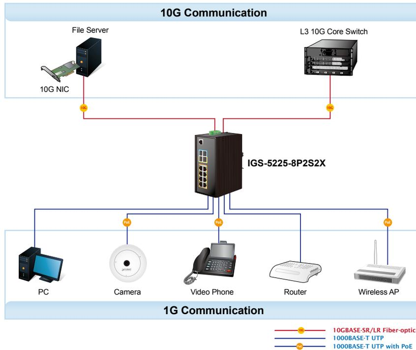
**Layer 3 VLAN Routing and 10G Uplink Application**
